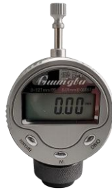
Figure 1 — Digital dial indicator forming part of the CSI roller-wave/flatness measurement system.
