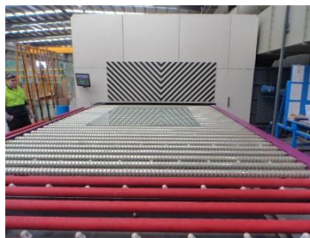
Figure 5 — Visual indication of roller-wave optical distortion in horizontally toughened glass. The glass is shown exiting the toughening furnace onto the roller bed. Distortion of the reflected zebra-board pattern provides a visual indication of changes in the glass surface profile.
